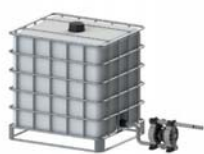
Pump installed below head (positive suction)
